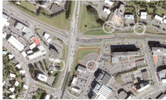
Location of geothermal wells
